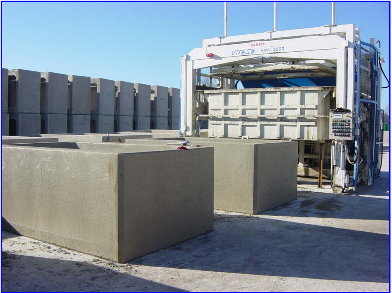
BOX CULVERTS PRODUCTION
