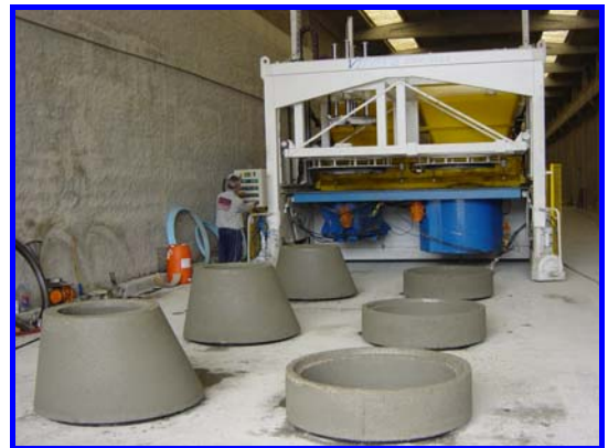
PIPES AND REGISTER CONES
